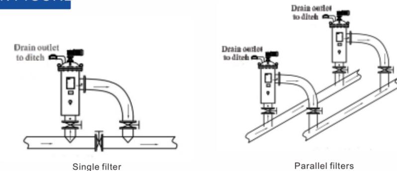
\* Note: the arrow in the diagram is the direction of flow. Vertical or horizontal installation and multiple parallel are available.
